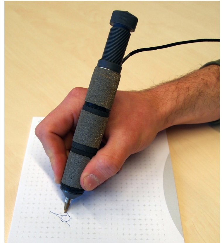
Tactile pen prototype using fabric-based sensors
